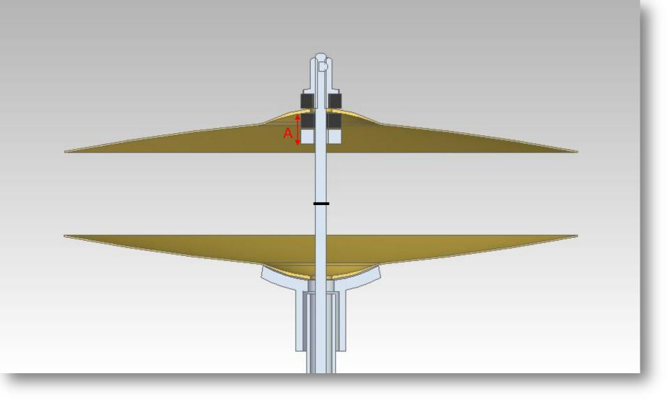
8- Measure the distance A from the bottom of the clutch to the top cymbal bell
