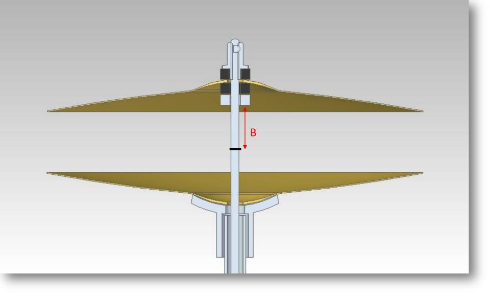
7- Measure the distance B from the bottom of the clutch to the pen's mark on the rod
