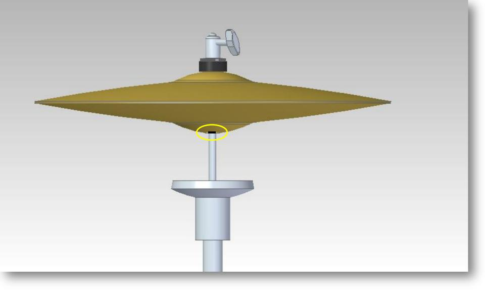
5- Keep the position and mark (with a pen) the hi-hat stand rod just below the bottom cymbal you are holding up
